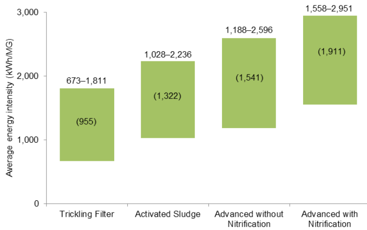
Figure 6: Energy Intensity of Wastewater Treatment Technologies in the United States (DOE 2012b)
