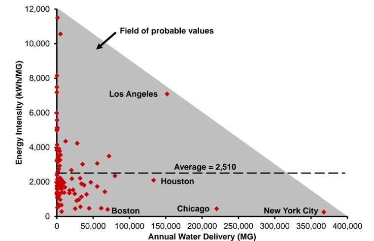
Figure 5: Energy intensity vs. water system size
