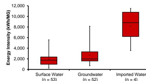
Figure 3: Energy intensity by primary water source type
